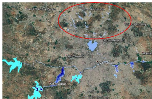
Fig. 1.15: A flood inundation map of Hyderabad city superimposed over the Google map.
