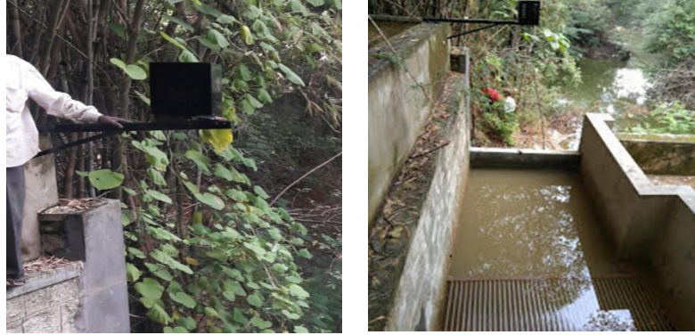
Fig. 1.11: Water level sensor installed at the outlet of the drainage network which is used for the rainfall runoff modelling of the IISc Catchment.
