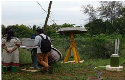
Fig. 1.18: The rainfall and level sensors developed by CDAC, Thiruvananthapuram.
